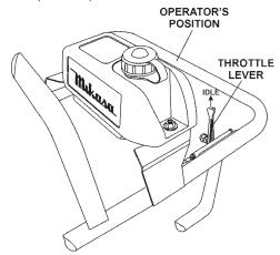
Figure 12. Throttle Lever (Idle)
